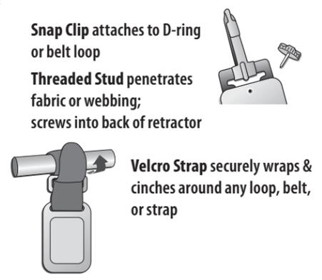
Snap Clip attaches to D-ring or belt loop
